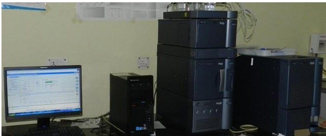
WATERS Acquity UPLC H-Class, Coupled with Acquity- TQD MS/MS
